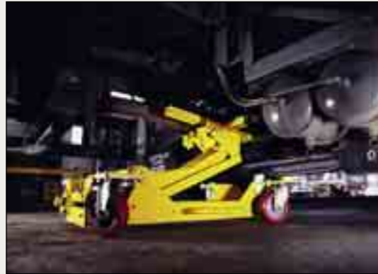
A versatile and indispensable tool when removing or fitting prop shafts, diffs, wheel drums and hubs.
